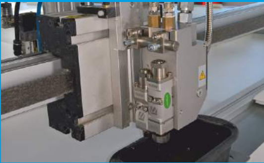
Hot melt applicator head HM-X* for precise bead and spray application.
