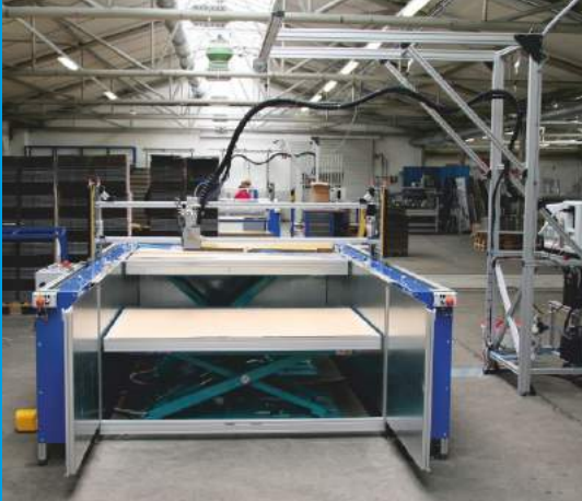
GLUEJET® PAI2 with integrated hydraulic lifting table: capacity 840 mm.
