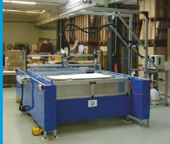
GLUEJET® PI2 with integrated electro-mechanic lifting table: capacity 350 mm.
