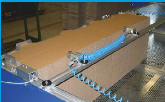
Repositioning cylinders fix the product for a precise glue application.
