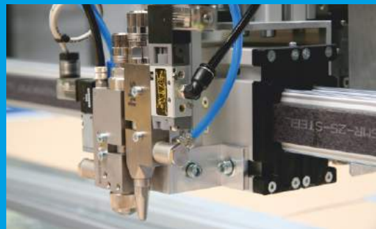
Cold glue applicator heads KR and KS* for hot/cold glueing in one cycle.
