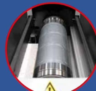
Full rotary die cut option. Enables the use of rotary dies from 12" (305mm) to 25½" (648mm).
