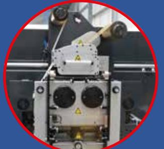
Flat bed hot foiling station with foil saver
